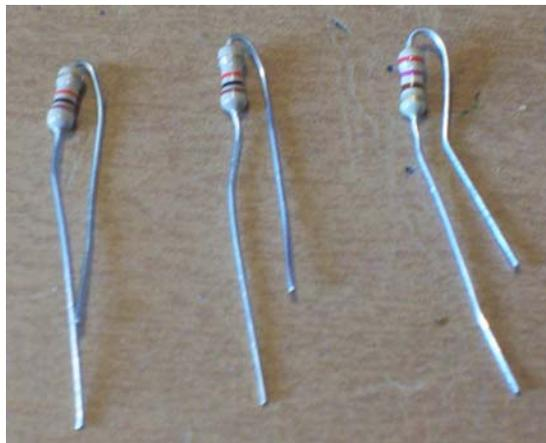
*The right way to bend resistor lead before soldering them.*
