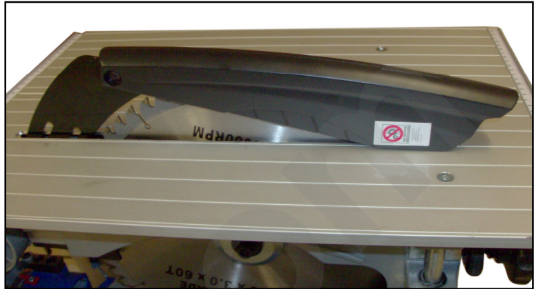
Figure 32 – Fixed and moveable guards.
