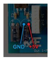
Most suitable sources of stabilized 5V supply for potentiometers are shown on the pictures on the left and right.
