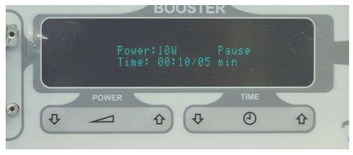
The operation can be continued by pushing the Start or the Continue button and can be aborted by pushing the Pause button. After the abort another treatment can be set and started.
