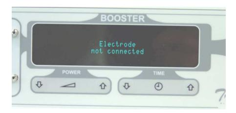
If the electrode is not correctly placed onto the patient or it's seriously damaged, a tuning error can occur.
