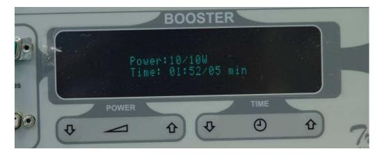
Both the time and power values can be changed during the operation by the Power-set and Time-set buttons.
