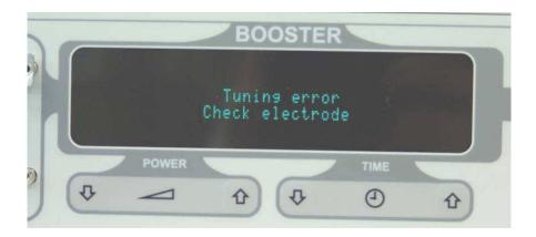
In this case you must be check the electrode itself and the position of the electrodes on the patient.
