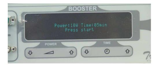
Here the parameters of action can be set by the Power-set and the Time-set buttons. After that the action can be started by pushing the Start button. In this case the device will use the last saved tuning position (see next point).
