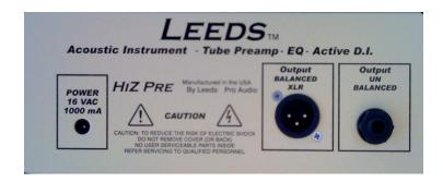
Unbalanced output – Buffered ¼ inch output to drive a monitor or stage amplifier. The buffer allows both the 1/4 and XLR outputs to be used simultaneously without loading down the output stage of the HiZ Pre. Cable Wiring:
