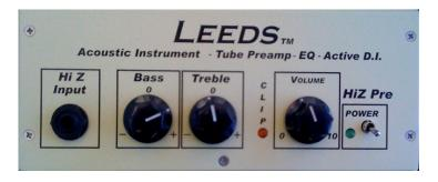
Hi Z input – High impedance input matched to piezo electric elements such as under saddle and soundboard transducers.
