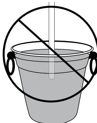
\* DO NOT ALLOW DRAINLINE TO BE SUBMERGED IN WATER
