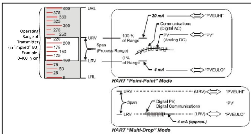
**Figure 1 – HART Point-to-Point and Multi-drop Value Scaling**
