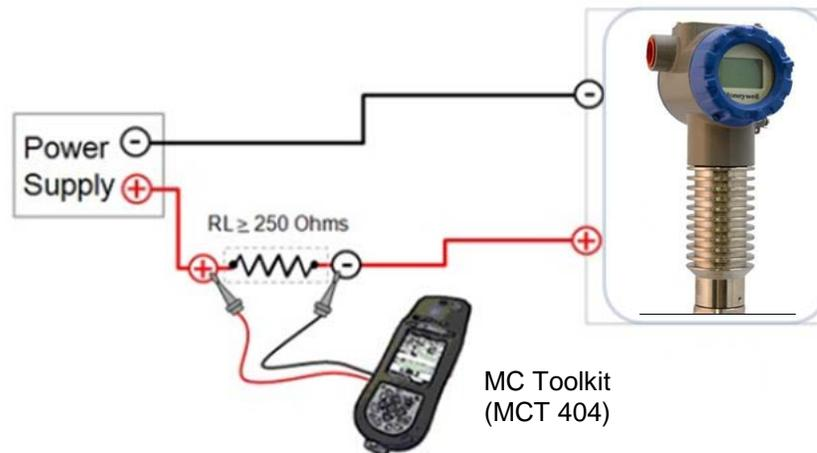
**Figure 2 – MC Toolkit-Transmitter Electrical/Signal Connections**
