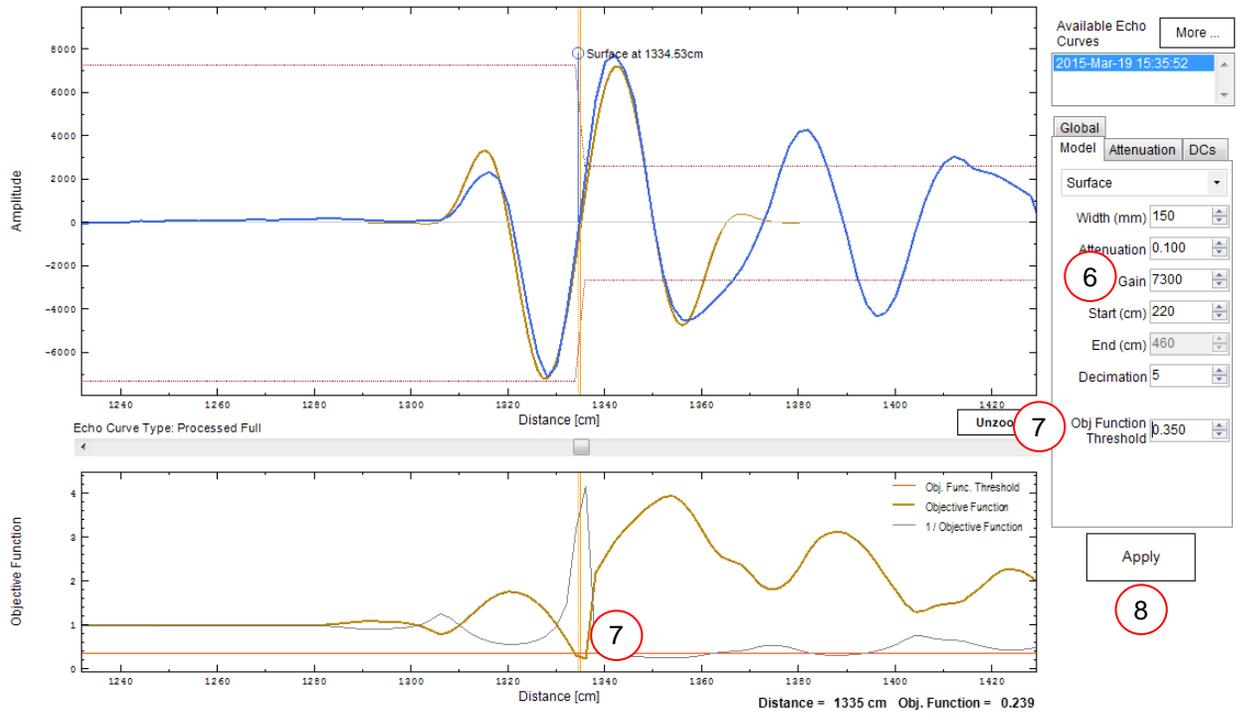
Next, go to Monitor and read a full echo curve. Check that the correct Reference, Surface and Interface measurements were found.
