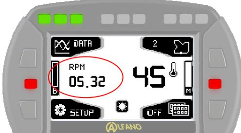
With RPM wire installed, the engine timer display will be replaced by the RPM data in real time.
