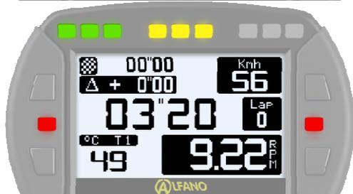
When starting the engine. The RPM data display « Layout » will be replaced from the « WELCOME » page to race mode, and the values of sensors are displayed in real time.
