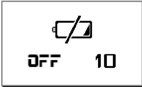
When this message displays, the PRO III will automatically turn off after 10 seconds.
