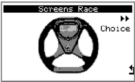
Press sequentially on « **Choice** » to scroll through the race displays (layout). You will have the choice of 5 different race displays.
