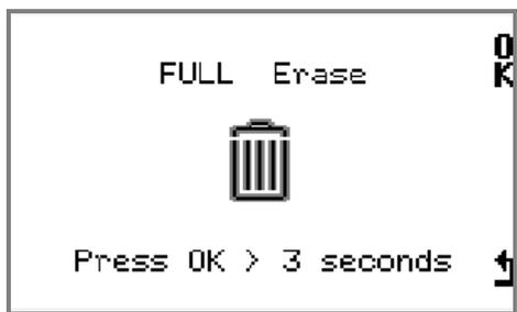
Press and hold for 3 seconds on « **OK** » to launch the procedure of memory erasing.
