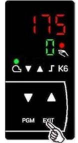
By design, the 0 output starts driving the modulating device to low fire, but if you promptly press the **▲** after the red LED above the hand icon turns on, you can prevent the from going all the way.
