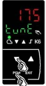
When **tunE** stops flashing on it's own **Auto-tune** is complete.
