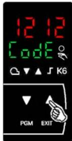
When the desired value is displayed, (and flashing), you can accept it by pressing **PGM** once, and releasing it.
