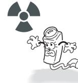
If exposed to radioactivity the CCD will fail.
