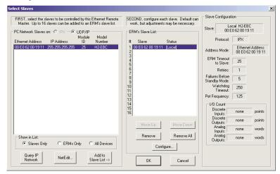
If the ERM or slave module is not on the list, try clicking on either the IPX or UDP/IP radio button (Query is automatically done when the protocol in the center column is changed). Confirm that your PC has IPX and TCP/IP protocol loaded.
