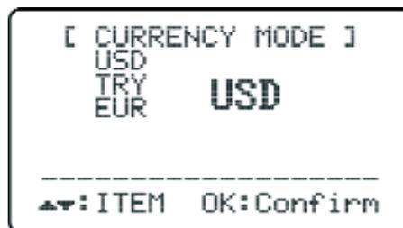
To change currency press «**CURRENCY**» button several times if necessary. Press «**OK**» button to save. Press «**CLEAR**» button to cancel.
