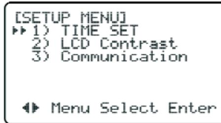
1 Present Time and date adjustments for results printing. For selector shifting use «▲», «▼», buttons «▲»,«▼», use «▶»,«◀» buttons to adjust.
