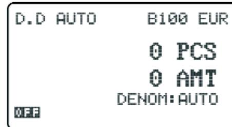
8.5 «**AUTO**» Sorting mode of the first orientation. In this mode counter sorts banknotes on the first banknote orientation (the one that was counted first):
