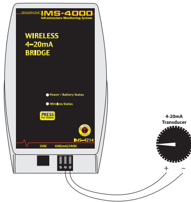
4-20mA Transducer using 24VDC power supply
