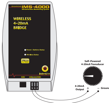
4-20mA sensor with self-powered transducer
