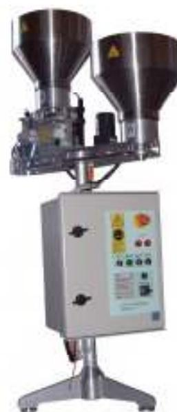
Figure 1 - SMA (Modular Feeding System)
