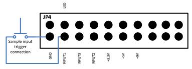
This figure shows the Input Header that is to the left of the network jacks on the main circuit board. You
