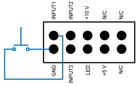
This figure shows the Input Header that is to the left of the network jacks on the Display Board. You can connect switches here to trigger standalone sequences or provide trigger events for interactive shows. See the *Stand Alone Operation* section for more information.
