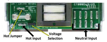
The Hot Input goes through the fuse. The Hot Jumper bypasses the fuse and should only be used when an external fuse is provided for the controller. Any of the Neutral Input tabs can be used to for the neutral input.
