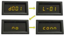
The Status Display rotates through four messages when the controller is powered but not connected to a controlling PC or Show Director and is not running a stand-alone sequence. It is displaying the LOR Unit ID, the DMX Universe address and "no conn" meaning no connection to any LOR network or DMX universe."
