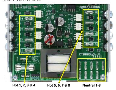
Note: Neutral wires can be placed in any of the neutral quick-connect blades on one side of the card.
