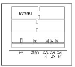
not possible to calibrate all three ranges because of limitations of the controls, readjust high voltage slightly and repeat steps 3, 4 and 5.
