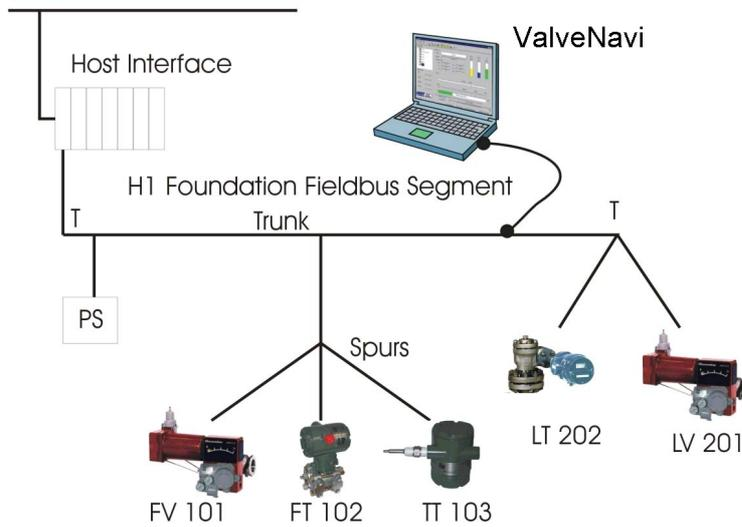
Figure 3.1 ValveNavi Reference Model Fieldbus Segment
