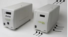
11.5.3 Always leave clearance for air flow between the X-Cite and walls or other equipment. Do not remove the rubber feet on the X-Cite unit or otherwise reduce/block the space between the bottom of the unit and bench top. This may compromise airflow through the unit.
