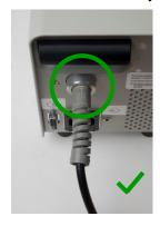
11.2.3 Always allow adequate clearance at the rear of the X-Cite unit and microscope to prevent excessive bending and/or crushing of the light guide against walls. Minimum bend radius to prevent immediate damage to the LLG is 40mm, however, a bend radius of at least 75mm is recommended for a light guide while "in use". Sharper bends can cause heat to build up and cause problems longer term.
