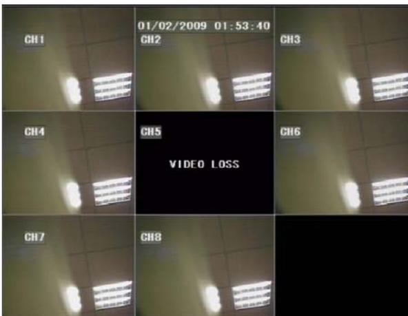
After initialization, the system will display main interface. When there are video inputs, live images from the cameras will be displayed on screen. You can use mouse to double-click the live image of any channel for full screen display; by double-clicking again, the display will return to display all cameras.
