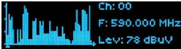
Results can be also displayed sorted by level (**pushing together SYNC and SCAN buttons**), making easier to pick up the best one.
