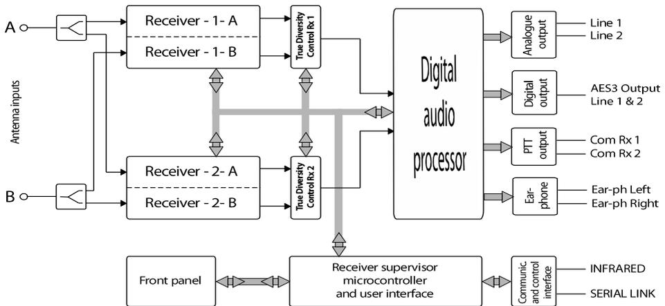
Above a schematic with an overview of main receiver functions.
