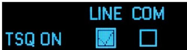
When tone squelch is on, output matrix between line and com (PTT) can be configured.
