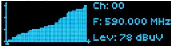
As per Wisycom standard, group 0 and group 9 are special; respectively the “center frequency” (474,482/... MHz) and the intergap frequency (i.e. 470/478/486/... MHz). A scan on group 0 will reveal in few seconds the overall DVB-T occupation on the area, while a scan on group 9 will give possible working frequency, usable also in presence of strong DVB-T signal (sort to speak working in the band-guard of 2 digital television channel).
