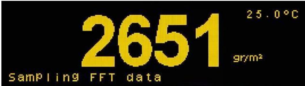
Illustration 25 - Display during FFT data acquisition
