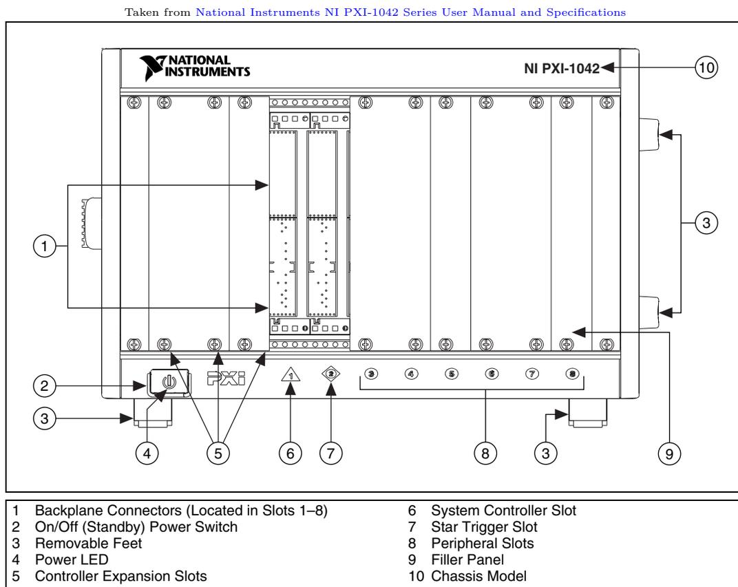
Figure 15: Front View of the PXI-1042 Chassis
