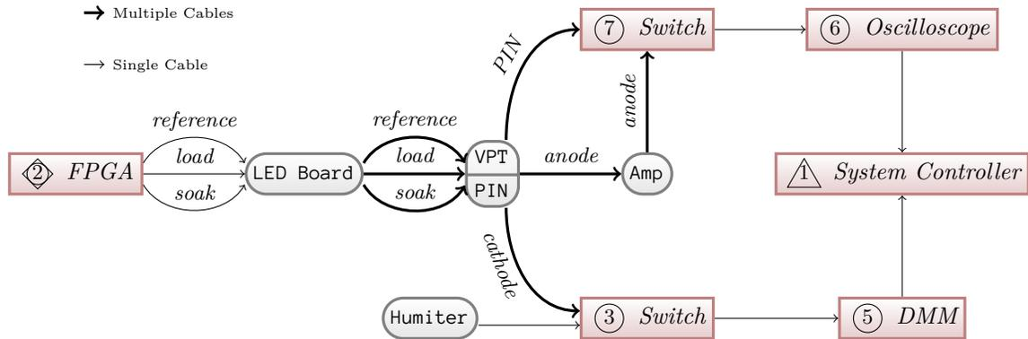
Figure 3: Signal Path in Teststand
