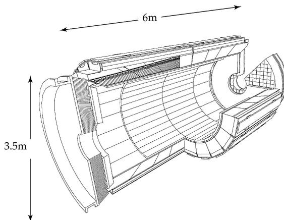
Figure 1: Schematic View of CMS Electromagnetic Calorimeter
