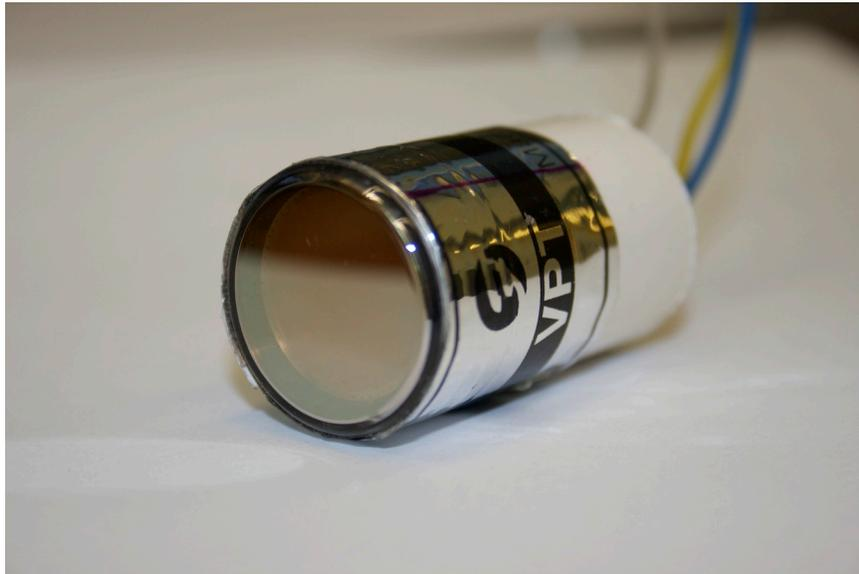
Figure 7: Photograph of Vacuum Photo-Triode
