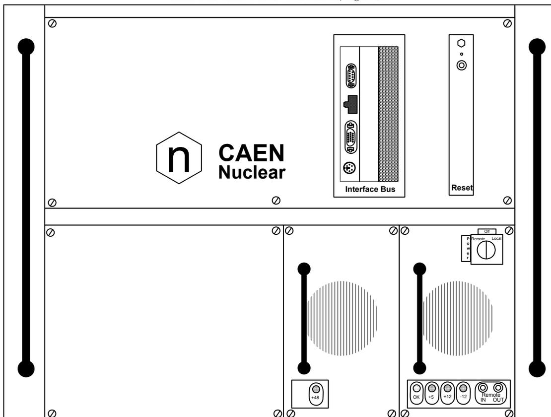
Figure 13: Front Panel of the SY1527LC System
