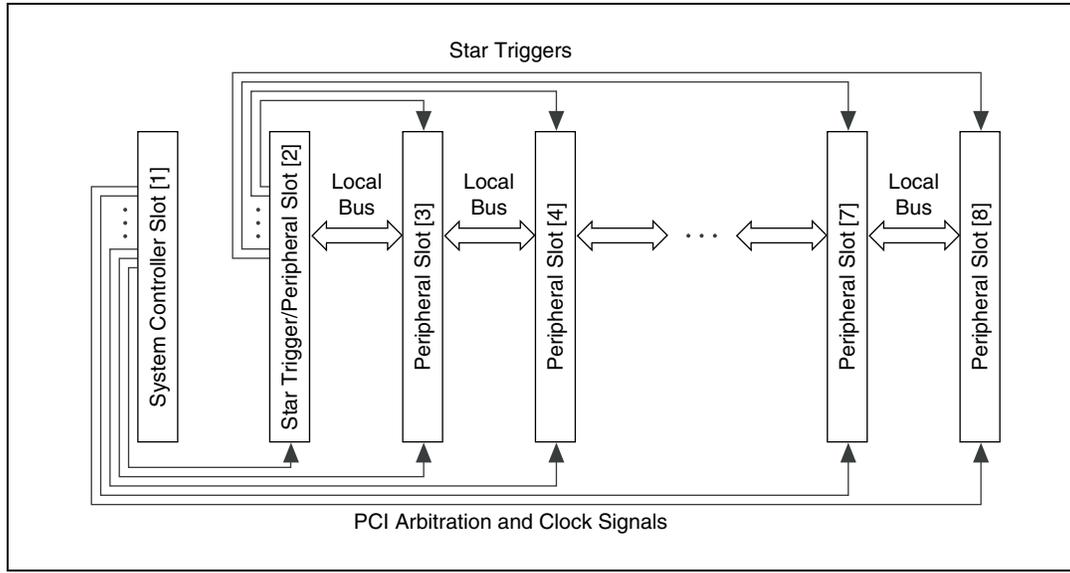
Figure 16: PXI Local Bus and Star Trigger Routing
