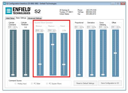
e. Increase the Proportional slider slowly (1% increments). The system should begin to move. If the system is not responding or is stuck in the fully extended or retracted position check tubing and feedback sensor polarity.
