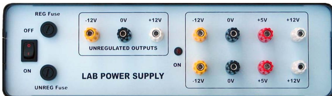
Figure 3: Front panel of the Mechatronics Lab bench power supplies.
