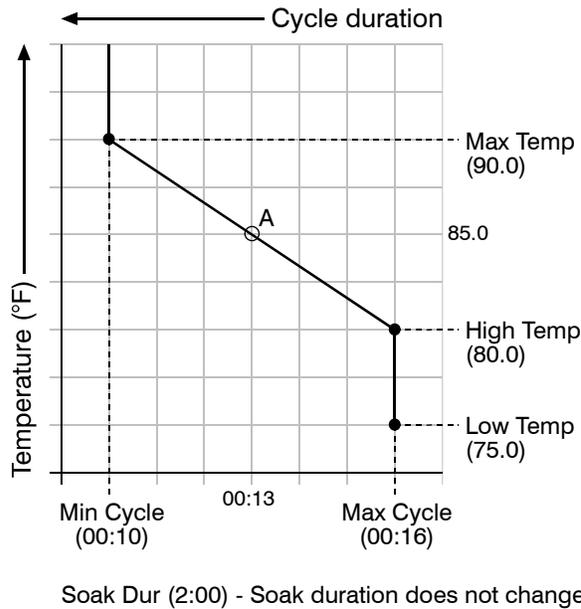
When the temperature is below the low temperature set point, no cooling cycle occurs.
