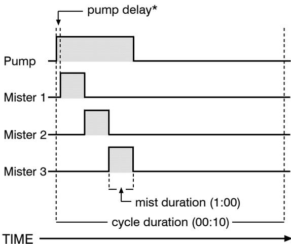
**Cooling cycle example when the temperature is at or above the maximum temperature set point**
