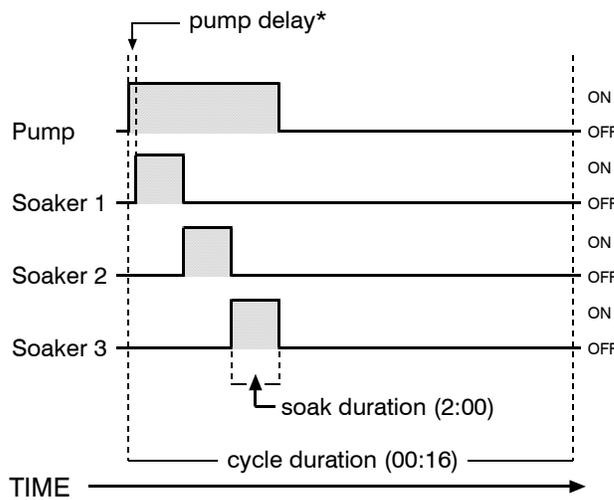
**Cooling cycle example when the temperature is at or above the maximum delay temperature set point**
