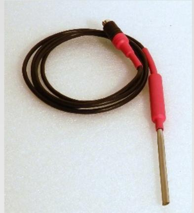
The MF300H+ is supplied with a Hall probe which is sensitive to magnetic fields. Flat, tangential probes measure the field through the flat surface. On special order, we can supply round, axial probes to measure the field along the axis of the probe (see Fig 1).
