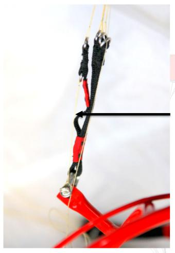
Fastening the risers works exactly in the same way as it has to be done for the soaring kit. The red mark has to be front-facing. Then please untie the knot which ties the brake line and the ring together and finally make sure the line goes through the ring freely.
