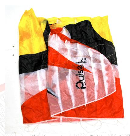
Finally put the risers back onto the wing and fold it 3 times in the other direction. The folding obtained should be about a hand wide so that it fits in its bag.
