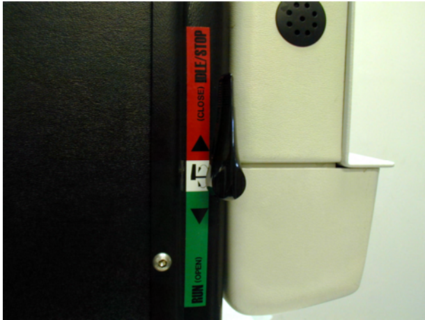
Figure 14: Manual Shutter Control Lever
