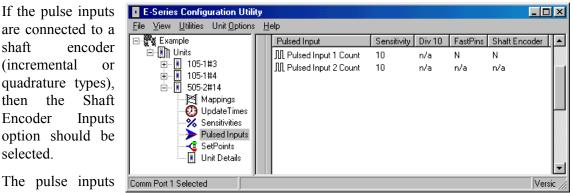
Sensitivity value. The pulse input sensitivity is the number of pulse increments since the last transmission to trigger another transmission. For example, if the pulse count at the last
