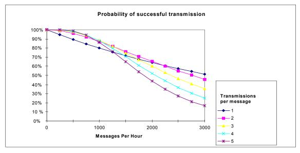
This assumes that the radio path is reliable and that there is no other radio users on this radio channel. If intermediate repeaters are used, then each repeated message should be counted as another message.
