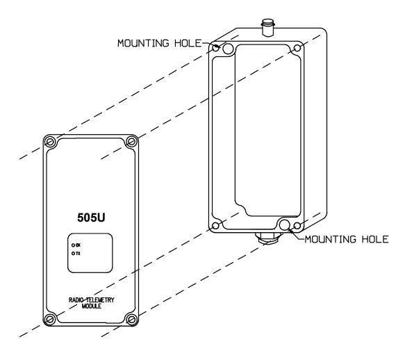
It is important to effectively earth the unit to help prevent radio noise and static electricity damage. The preferred method is to earth the module using the mounting screws to connect to an earthed surface. If this is not possible, use an earth lug in the mounting screw connection and secure the other end of the wire to a good earth.
