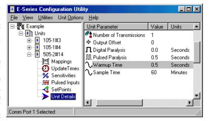
of the input. The warmup time allows the transducer to stabilise and become accurate after the loop supply is turned on.
