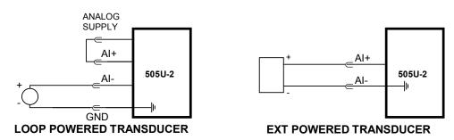
Loop powered transducers must be suitable for low voltage operation. Loop voltage available for the transducer is 8.5V for 505U-B modules and 1.5V less than the power supply voltage for 505U-E modules.
