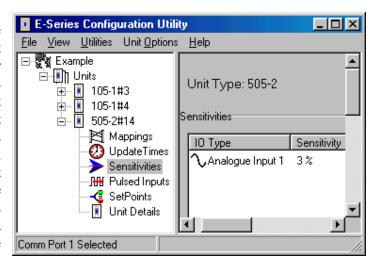
Each 1% corresponds to 0.2mA of signal. The sensitivity should be set to be greater than the natural "signal noise" of the analogue input. For example, if there is a signal oscillation of 1% on the input, then a sensitivity of less than 1% will result in continuous change transmissions which could overload the radio channel.
