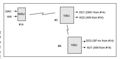
The setpoint status of the 505U is mapped (inverted) to DO3 of 105U#14, using 105U#13 as a repeater. The 505U AI is also mapped to AO1 of this module. That is, the AI is mapped twice.
