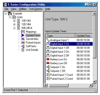
state. If the digital input is an alarm, then a user may wish the input to be updated more frequently when in the alarm state than when not in the alarm state. The analogue input and pulsed inputs only have one update time value.
