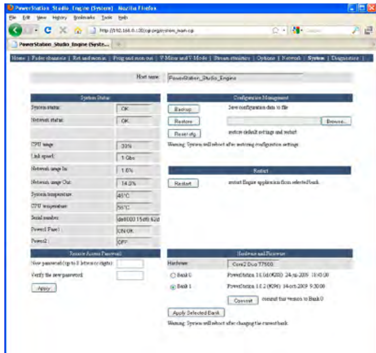
Fig. 10-5: PowerStation MixEngine System screen
