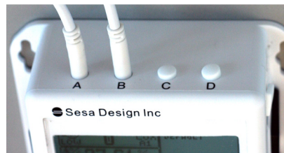
FIGURE 4b Sensor eUnits ports on the top of the iFarm controller
