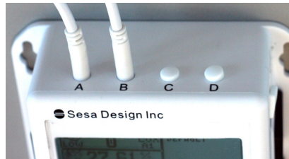
FIGURE A1.3.1 Sensor eUnits ports on the top of the iFarm controller
