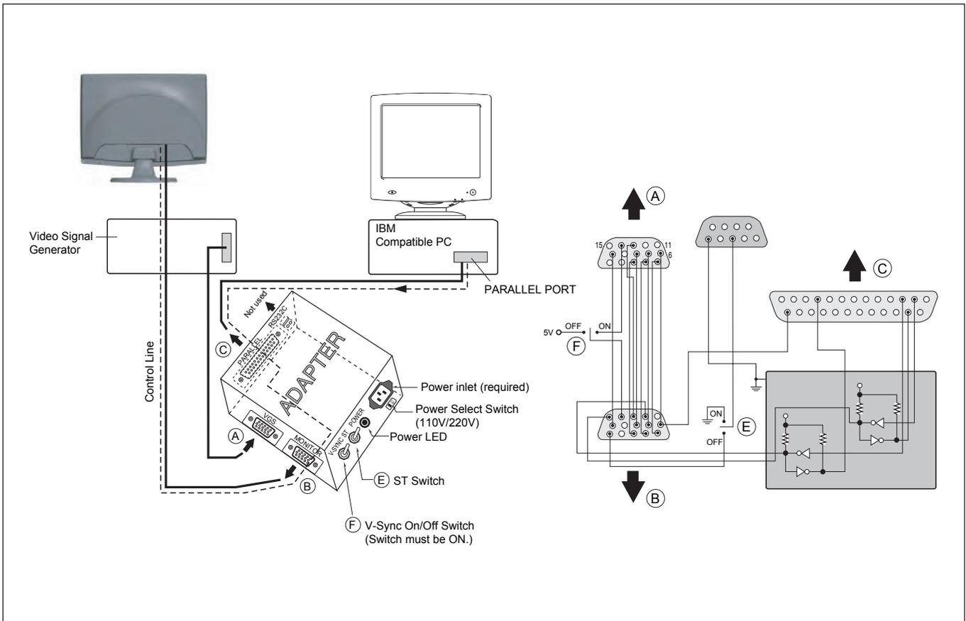
Figure 1. Cable Connection
