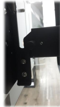
④ LCD panel is released from the hook lock.
