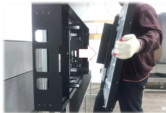
② Take the LCD panel assembly out with special care.
