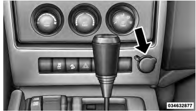
Front Power Outlet
