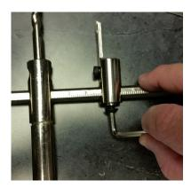
Figure 5 shows each blade holder set to the 4" mark. Although each blade holder is only 2" from the center of the tool, the diameter of the hole will be 4".
