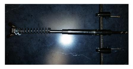
Slip the cutter shaft through the ball-bearing collar in the dust shroud (Fig. 2)
