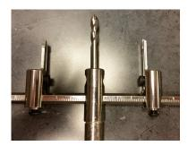
Using the included hex key, remove the stop screw from the end of the mounting bar (Fig. 7).
