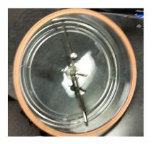
Slide the spring over the cutter shaft and secure with the wing-nut (Fig. 3)
