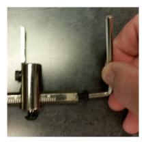
Loosen the set screw at the top of the blade holder and slide the blade holder off the mounting bar (Fig. 8).
