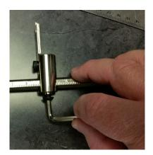
Remove the retaining screw from the blade holder and remove the blade (Fig. 9).
