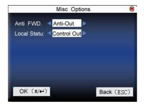
The choice of Machine models: Press ▲/▼ to switch the input box. Press ▲/▶ to modify the setting. Select Anti-Out, refer to out anti-pass back, only user's last record is in-record, can the door be open. Otherwise it will trigger the alarm signal as illegal access. Select None, refer to no anti-pass back, and no alarm will be triggered. After setting, press **Menu** directly to return to the last interface. Press "ESC" to cancel setting and return to the last interface.
