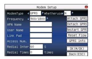
Scroll ▲ / ▼ key switch box or enter the cursor to the button to start the T9 input method type APN name or user name, the other way that through the input box scroll ◄/► button to select the items need to, or directly type a numeric value. After the set directly press М/← / "OK" (F7) button to save your settings and return on an interface, press the "ESC" (F8) to cancel and return to previous interface.
