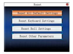
Press ▲/▼ to move cursor to the button to be operated. Press **OK** to start operation. The device will say "Are you sure to execute the current operation?" Press **OK** to reset it to factory state and press "**ESC**" to cancel operation.
