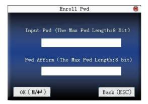
Input password (1 $\sim$ 8) according to device's prompt, and press **OK** to verify it. Then press **OK** save it or press **ESC** to exit without saving it.
