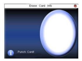
Put the card in the induction area, waiting for device to delete all the information in the card. If the card data has been stored in the device, the device will remind you whether to delete the information in the device or not. "Yes" is to delete the user's fingerprint and information in the device. "No" is to keep the information.
