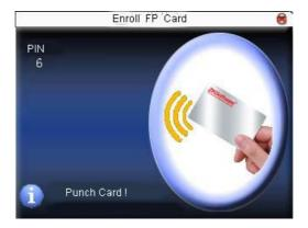
Step 5: Put the card in the induction area, waiting for the device to read fingerprint data into card until the enrollment succeeds.
