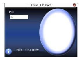
Step 2:Use keyboard to input the number to be enrolled (if the number has been there already, the device will prompt you to copy the information to the card.) ,and then press **OK**. The device will prompt you to move off your finger.
