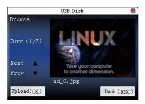
Insert U disk into USB slot of device. Press " $\blacktriangle/\blacktriangledown$ " to preview the pictures of U disk. If you want to upload the picture, click **OK**. Then the next picture will appear automatically. After upload, press ESC to exit.
