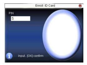
Step 2:press keyboard to input the number to be enrolled (if the number has been there already, the device will prompt you to copy the information to the card.) ,and then press  $\mathbf{OK}$ .
