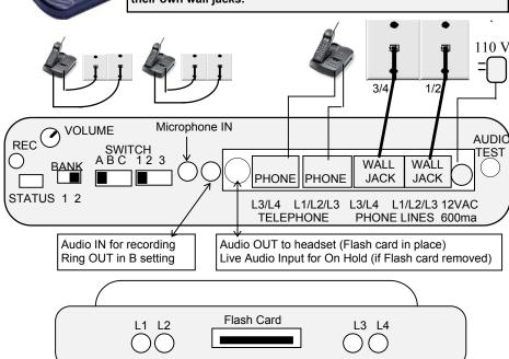
**Connection Test:** To confirm that everything is connected correctly, select line 1 on the phone, confirm that L1 Red LED on SX8600 (left most LED) turns ON, then press the L1 Audio Test button to hear the audio. Double check your connections or adjust the volume if needed.
