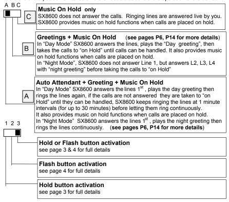
Regular 1 to 4 line telephones have differences when it comes to Music-On-Hold activation compatibility, some models work by just pressing HOLD button some work via Flash then Hold, this switch lets you find out which setting works best for your telephones.
