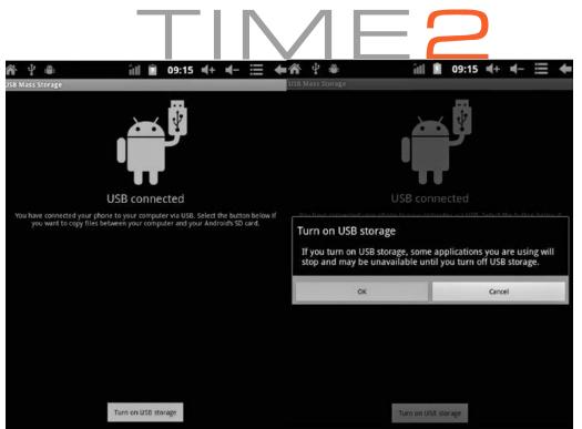
Step 4: Please press "turn on USB storage". Then you will find the follo wing photos: Please choose "OK". Then USB is connected. "USB is connected": means external memory (SD) loading is completed, and you can see the correspon ding letter in the PC terminal.
