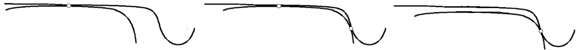
Fig.8.45. Types of contact for a pair of profiles allowing two-point contact: one-point contact, two-point contact and creeping up
