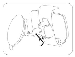
• To release the Parrot MINIKIT Smart, press the release buttons on the craddle.
