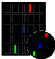
Cluster pixel defect type 3a Sub-pixels/dots in a cluster area constantly lit
