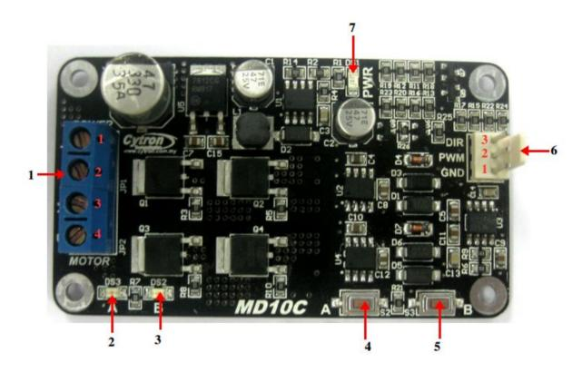
1. Terminal Block – Connect to motor and power source.
