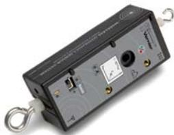
The Wireless Dynamics Sensor System (WDSS) allows you to take data from a three-axis accelerometer, force sensor, and altimeter, using a Bluetooth® wireless connection to your computer. It is the perfect tool for dozens of physics and physical science experiments such as:
