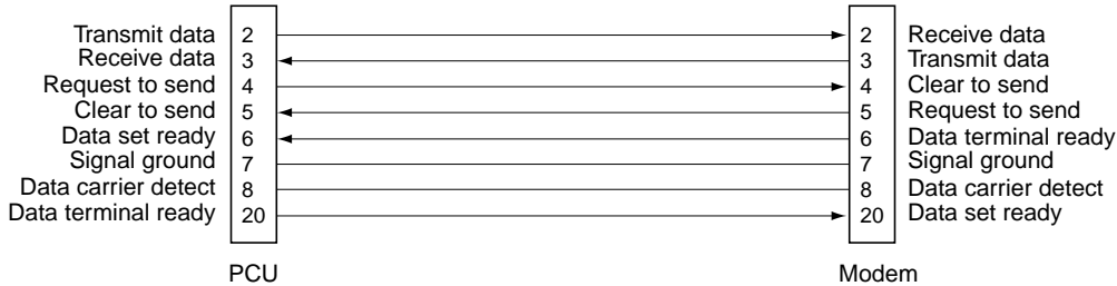
Figure 3-5 PCU-to-Modem Cable Configuration
