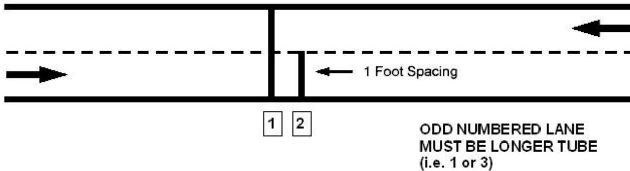
**Directional** This road tube configuration is used for counting two-way traffic on a narrow road. A road tube pair (such as 1-2 or 3-4) is laid out across both lanes of a road one foot apart. The Unicorn Limited will determine (from the order of actuation) the proper directional count for each lane.
