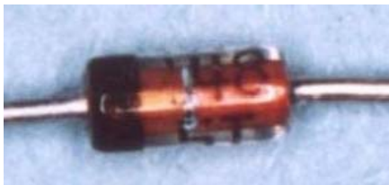
1N914 signal diode
