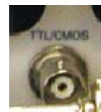
Sync output of function generator
