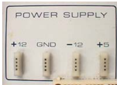
Figure 4-5. Power supply on prototyping board (left). Connect these using wires to the strips sketched on the right for convenient use.
