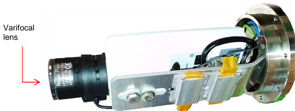
Abb.6.11 – Mounting adapter with installation components
