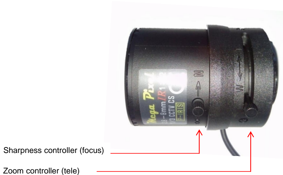
Figure 6.12 – Mechanical adjustments at the lens
