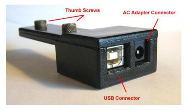
The Multifunction Attachment (called the "Attachment" below for simplicity's sake) allows for a variety of functions, including:
