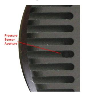
The pressure sensor aperture allows the pressure sensor to come in direct contact with the surrounding water and measure the hydrostatic pressure.
