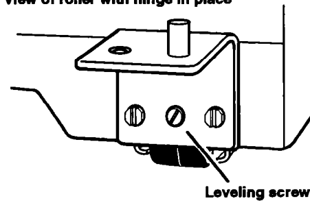
View of roller with hinge in place
