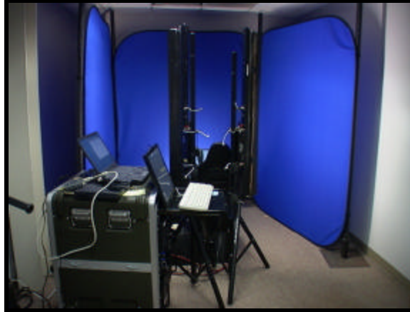
Figure 5. VEHELO Portable Mock Cockpit and Matting
